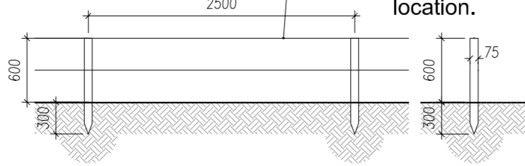
TYPICAL ELEVATION DETAIL SD103 A - 600mm POST AND WIRE FENCE scale 1:50
